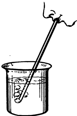
FIG. 202. — Water does not enter the tube as long as we blow into it.
